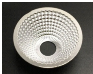
Size: 50.0*15.9mm Model: AHR5016D/15G/24G/36G/45G Beam angle: 15°/24°/36°/45° Material: PC+Coating Efficiency: >88%
