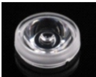
Size: 19.5*6.2mm Model:ABL19D620 Beam angle: 35° Material: PMMA Efficiency: >93% LED type:SMD3528;SMD3030
