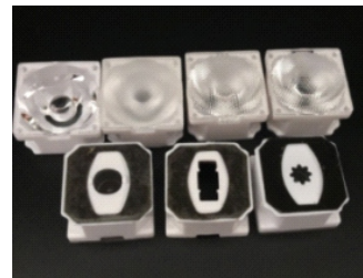
Size: 21.6*12.0mm Model: AYS216D/10G/15G/30G/60G Beam angle: 10°/15°/30°/60° Material: PMMA Efficiency: >90%
