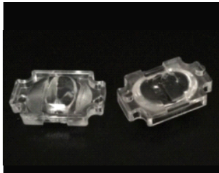
Size: 14.6*9.6mm Model: ALST14D13565G Beam angle: 135°*65° Material: PC Efficiency: >88%
