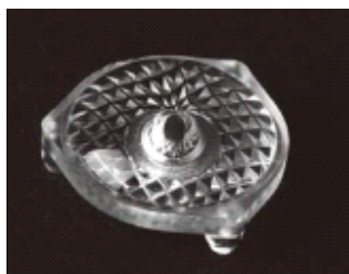
Size: 15.5*5.49mm Model:ATV15D549 Beam angle: 175° Material: PMMA Efficiency: >93% LED type:SMD3528
