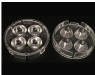
Size: 35.2*7.4mm Model: AS04H35D/24G/35G Beam angle: 24°/35° Material: PMMA Efficiency: >90%
