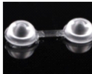
Size: 32.7*11.7*5.18mm Model: ABL32D518 Beam angle: 150° Material: PMMA Efficiency: >93% LED type:SMD5050
