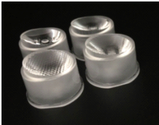
Size: 22.5*12.4mm Model: AMS22DA/10G/25G/40G/1045G Beam angle: 10°/25°/40°/10°/45° Material: PMMA Efficiency: >90%
