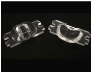
Size: 22.0*9.0mm Model: ADST22D13070G Beam angle: 130°*70° Material: PC Efficiency: >88%
