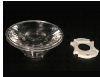
Size: 60.0*22.2mm Model: AHC0B60DH/12G/24G/38G Beam angle: 12°/24°/38° Material: PMMA Efficiency: >90%
