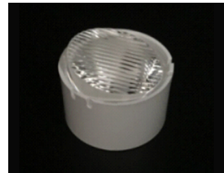
Size: 20.8*12.7mm Model: AJS21D1535GA Beam angle: 15°*35°asymmetric Material: PMMA+PC Efficiency: >90%
