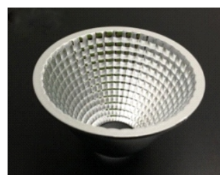
Size: 75.0*27.0mm Model: AHR75DL/15G/36G Beam angle: 15°/36° Material: PC+Coating Efficiency: >88%
