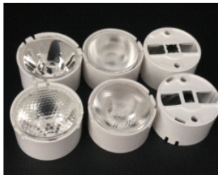
Size: 20.8*12.7mm Model: AJS21D/10G/15G/25G/35G Beam angle: 10°/15°/25°/35° Material: PMMA+PC Efficiency: >90%
