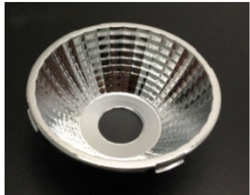
Size: 84.0*31.3mm Model: AHR84D15G/24G/36G Beam angle: 15°/24°/36° Material: PC+Coating Efficiency: >88%
