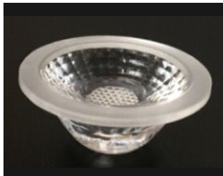
Size: 47.5*20.0mm Model: AHC0B47D35G Beam angle: 35° Material: PMMA Efficiency: >90%
