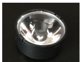
Size: 29.0*15.0mm Model: AYS29D5G Beam angle: 5° Material: PMMA Efficiency: >90%
