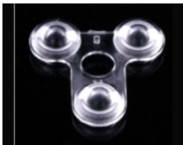
Size: 33.0*33.0*5.2mm Model: ABL33D520 Beam angle: 150° Material: PMMA Efficiency: >93% LED type: SMD5630
