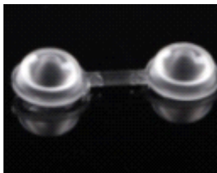
Size: 33.0*33.0*5.2mm Model: ABL33D587 Beam angle: 90° Material: PMMA Efficiency: >93% LED type:SMD5630
