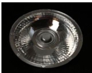
Size: 50.0*8.6mm Model: AHCOB50D12G Beam angle: 12° Material: PMMA+COATING Efficiency: >90%
