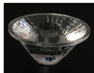
Size: 41.3*22.2mm Model: AHC0B41D15G/24G/38G/60G Beam angle: 15°/24°/38°/60° Material: PMMA Efficiency: >90%
