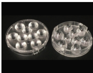
Size: 35.2*7.4mm Model: AH09H35D/24G/35G/45G Beam angle: 24°/35°/45° Material: PMMA Efficiency: >90%
