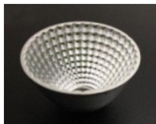
Size: 60.0*35.2mm Model: AHR60D36G Beam angle: 36° Material: PC+Coating Efficiency: >88%
