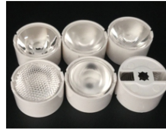
Size: 21.0*12.35mm Model: AMS21D/15G/25G/35G/60G/90G Beam angle: 15°/25°/35°/60°/90° Material: PMMA+PC Efficiency: >90%
