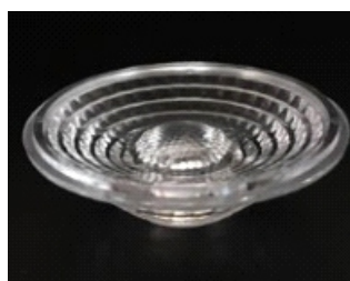
Size: 41.8*12.24mm Model: ADCOB41D/38G/60G Beam angle: 38°/60° Material: PMMA Efficiency: >90%
