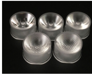
Size: 22.5*12.4mm Model: AMS22D/10G/25G/30G/40G/60G Beam angle: 10°/25°/30°/40°/60° Material: PMMA Efficiency: >90%
