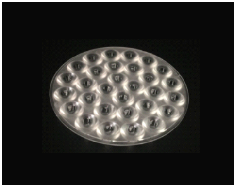
Size: 65.0*7.3mm Model: AH30H65D/15G/24G Beam angle: 15°/24° Material: PMMA Efficiency: >90%
