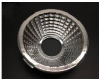
Size: 65.0*23.2mm Model: AHR65D/15G/36G Beam angle: 15°/36° Material: PC+Coating Efficiency: >88%
