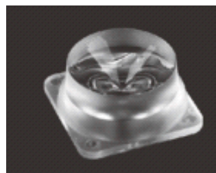
Size: 15.0*7.0mm Model: ATV15D700 Beam angle: 175° Material: PMMA Efficiency:>93% LED type: SMD3528;SMD3030
