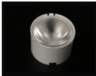
Size: 21.0*12.8mm Model: ADS21D20G Beam angle: 20° Material: PMMA+PC Efficiency: >90%
