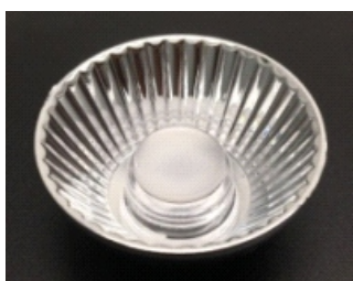
Size: 38.0*13.9mm Model: AHR38D/24G/36G Beam angle: 24°/36° Material: PC+Coating Efficiency: >88%
