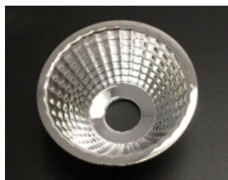
Size: 50.0*17.5mm Model: AHR5017D/15G/36G Beam angle: 15°/36° Material: PC+Coating Efficiency: >88%
