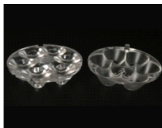
Size: 32.0*7.5mm Model: AH06H32D/12G/24G/45G Beam angle: 12°/24°/45° Material: PMMA Efficiency: >90%
