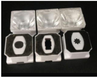
Size: 21.6*12.0mm Model: AYS216D/1035G/1045G/1060G/1245G Beam angle: 10°/35°/10°/50°/10°/60°/12°/45° Material: PMMA Efficiency: >90%
