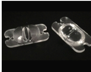
Size: 19.0*9.6mm Model: ALST19D13555G Beam angle: 135°*55° Material: PC Efficiency: >88%
