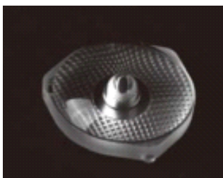
Size: 15.53*5.73mm Model:ATV15D573 Beam angle: 175° Material:PMMA Efficiency: >93% LED type:SMD3528;SMD3030
