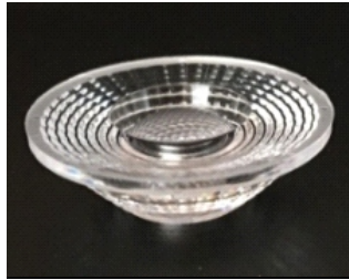
Size: 35.0*9.8mm Model: ADCOB35DL45G Beam angle: 45° Material: PMMA Efficiency: >90%
