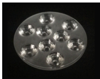
Size: 44.0*8.5mm Model: AH09H44D/24G/38G/45G Beam angle: 24°/38°/45° Material: PMMA Efficiency: >90%
