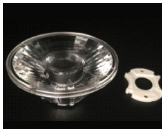
Size: 75.0*32.0mm Model: AHCOB75DH/12G/24G Beam angle: 12°/24° Material: PMMA Efficiency: >90%
