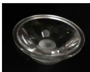
Size: 60.0*28.0mm Model: ADC0B60D/15G/30G/60G Beam angle: 15°/30°/60° Material: PMMA Efficiency: >90%
