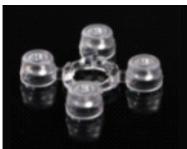
Size: 31.5*25.6*6.68mm Model: ABL31D668 Beam angle: 90° Material: PMMA Efficiency: >93% LED type: SMD3528
