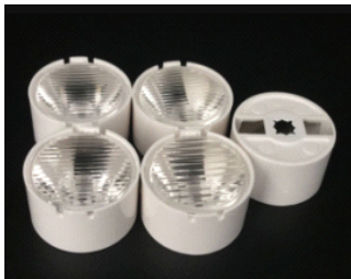
Size: 21.0*12.35mm Model: ADS21D/1030G/1045G/1065G/1090G Beam angle: 10°*30°/10°*45°/10°*65°/10°*90° Material: PMMA+PC Efficiency: >90%
