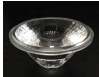
Size: 43.0*22.5mm Model: ADC0B43D/24G/38G/60G Beam angle: 24°/38°/60° Material: PMMA Efficiency: >90%
