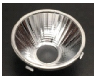
Size: 46.5*19.1mm Model: AHR46D/15G/24G/36G Beam angle: 15°/24°/36° Material: PC+Coating Efficiency: >88%
