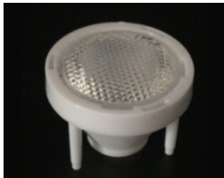
Size: 23.4*16.0mm Model: AYS23D/25G/40G Beam angle: 25°/40° Material: PMMA+PC Efficiency: >90%
