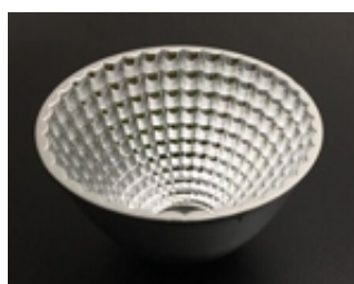
Size: 65.0*20.7mm Model: AHR65DL/15G/24G/36G/45G Beam angle: 15°/24°/36°/45° Material: PC+Coating Efficiency: >88%
