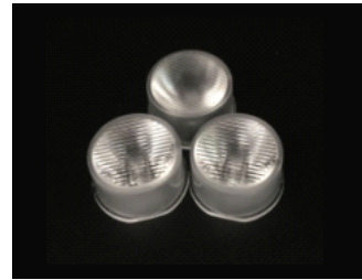
Size: 22.5*12.4mm Model: AMS22D/1045G/1065G/2065G Beam angle: 10°/45°/10°/65°/20°/65° Material: PMMA Efficiency: >90%
