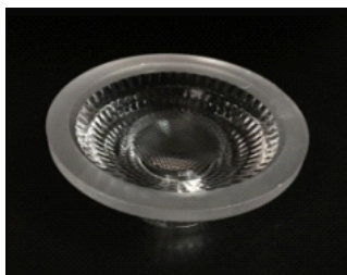
Size: 60.0*25.0mm Model: AGCOB60D/38G/45G/60G Beam angle: 38°/45°/60° Material: PMMA Efficiency: >90%
