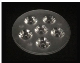
Size: 44.0*8.5mm Model: AH06H44D/24G/38G/45G Beam angle: 24°/38°/45° Material: PMMA Efficiency: >90%
