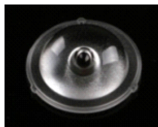
Size: 24.4*7.25mm Model:ABL24D725 Beam angle: 160° Material: PMMA Efficiency: >93% LED type:SMD LED4PCS
