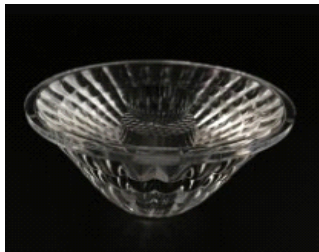
Size: 58.0*31.6mm Model: AHC0B58D/24G/38G/60G Beam angle: 24°/38°/60° Material: PMMA Efficiency: >90%
