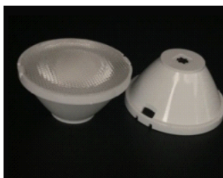
Size: 37.0*18.45mm Model: AMS37D Beam angle: 60° Material: PMMA+PC Efficiency: >90%
